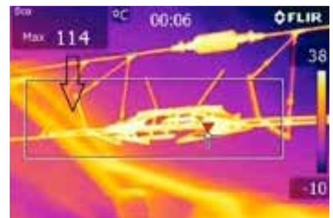
*Early detection of rises in temperature helps DMRC to prevent costly failures and downtime.*
